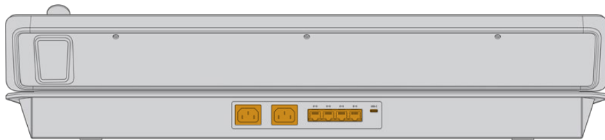
ATEM 2 M/E Advanced Panel rear connectors
