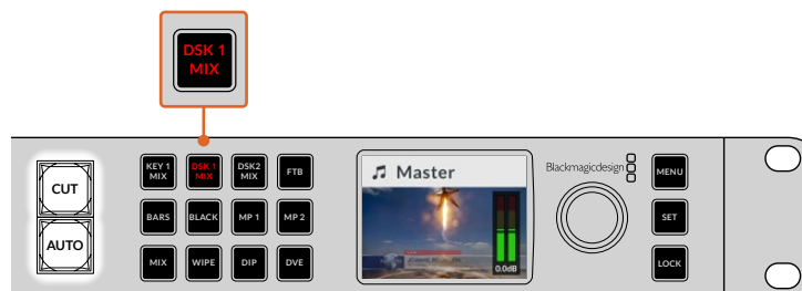
Press the DSK 1 MIX button to fade the downstream key 1 on and off air
